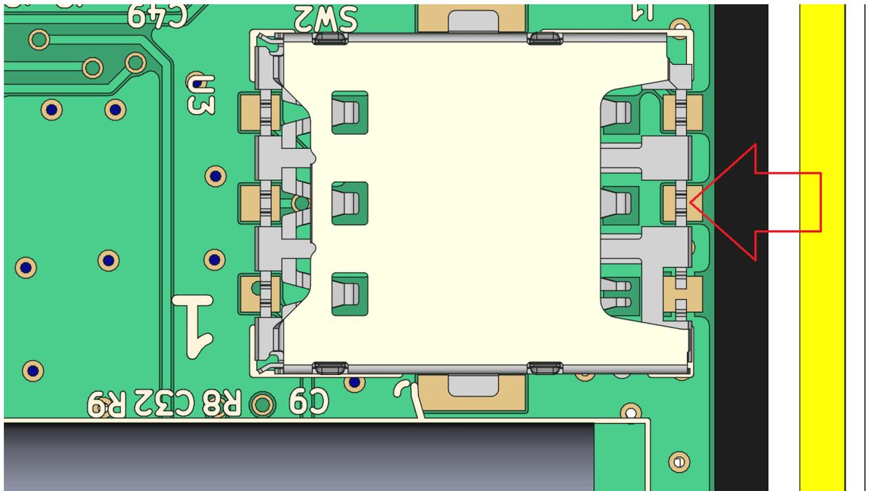
2. Next use the index finger to slide the sim all the way out. If you are facing any difficulties in removing the sim please feel free to contact us.
