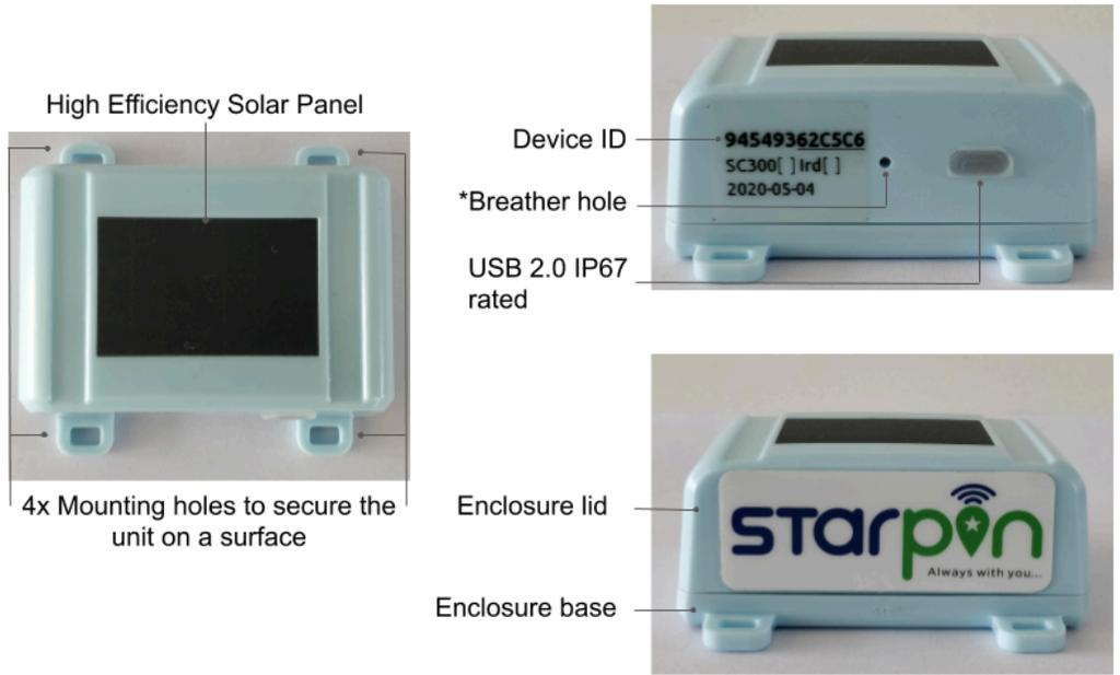
**\*Do not insert anything into the breather hole. Punching the breather hole membrane will cause water intrusion problems and will void warranty.**
