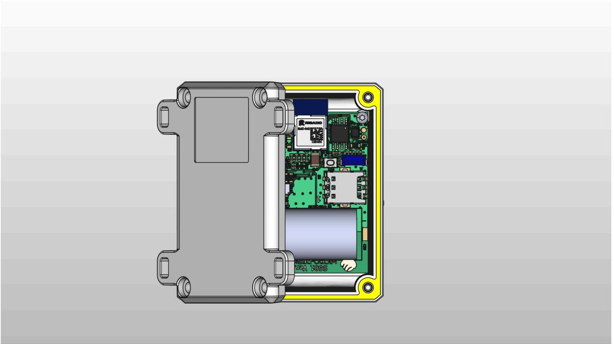
3. Locate the SIM holder. It's position is at the center of the board on the longer edge away from the USB.
